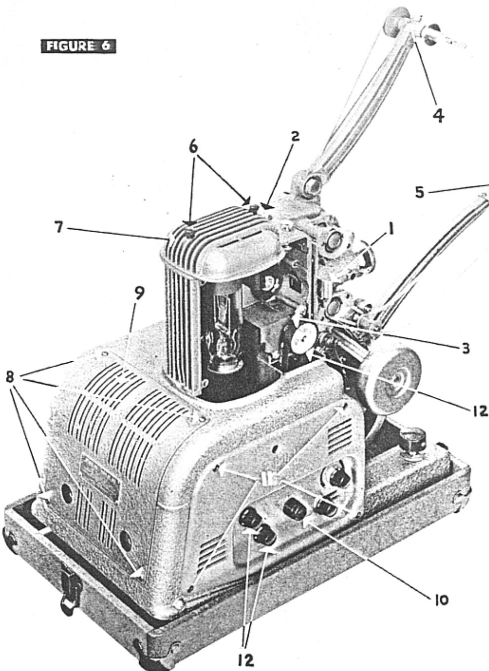
b. After each 75 hours of operation apply 2 or 3 drops of oil to the spindle oilholes (4 and 5 Fig. 6).
